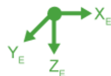
Earth-Fixed (Inertial) Coordinate System (Z-Down)
